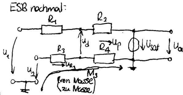
~~$u_d = u_p - u_2 + u_2 - u_1 + i_1 R_1 = u_p - u_1 + i_1 R_1$~~
