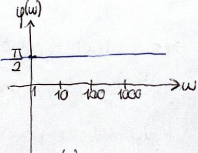
•  $H(j\omega) = \frac{1}{j\omega} = \frac{-j}{\omega} \Rightarrow v(\omega) = 20 \log \frac{1}{\omega} = -20 \log \omega$
